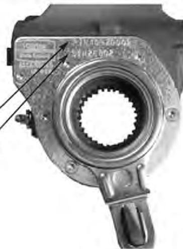
Reference The O.E. Part Number That Is Stamped Into The ABA Side Cover To The 400 Series Replacement Service Number Below.
